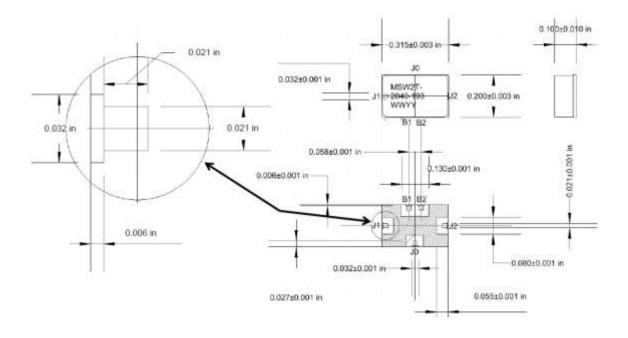
Note: Metalized area on backside is the RF, DC and Thermal ground. In user's end application this surface temperature must be managed to meet the power handling requirements.
